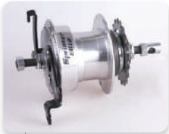
1995 AT5 5-Speed Drum Brake
