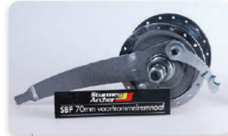
1977 SBF Front Drum Brake
